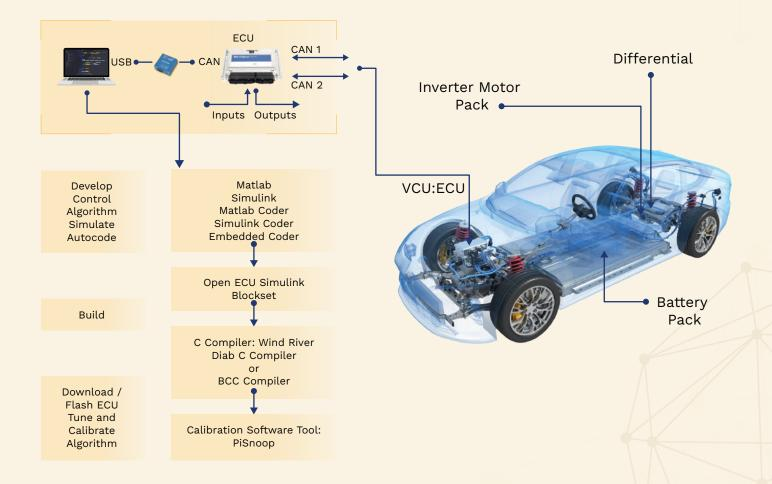
The Embedded Software Development for the VCU (for that matter, for any ECU) are as follows:
